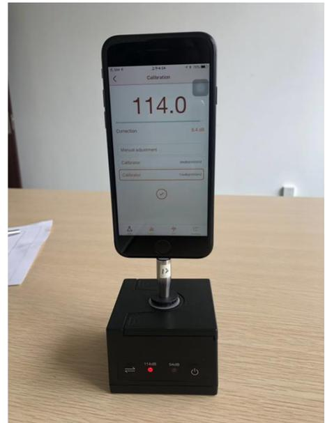
**Manual Adjustment:** Manually set the Sound Pressure Level according to the calibrator
