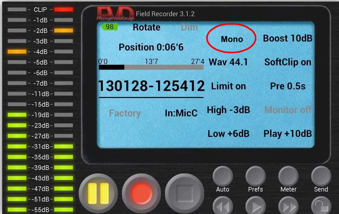
Figure 2: Screenshot of the *Pfitzinger Voice Design* field recorder. The *Mono* setting has to be used instead of *Stereo*.
