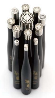
What's in the N series Box: The N series are delivered in a hard shell plastic transport case Including a professional shock mount, wind screen and frequency test report.
